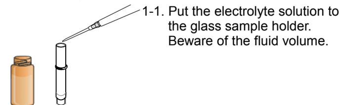
1-1. Put the electrolyte solution to the glass sample holder. Beware of the fluid volume.
