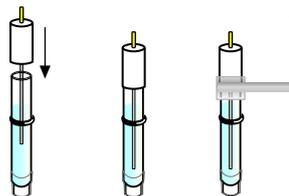
1-2. Insert the RE-7S Teflon cap into the glass holder, and fasten the cap tightly. Seal the cap to avoid evaporating of the inner solution.
