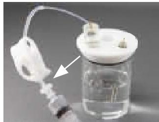
Leave the tubing clamp at open state. Use the disposable syringe and suction the acidic solution gently till the solution is near the female lure fitting and close the tubing clamp firmly.
